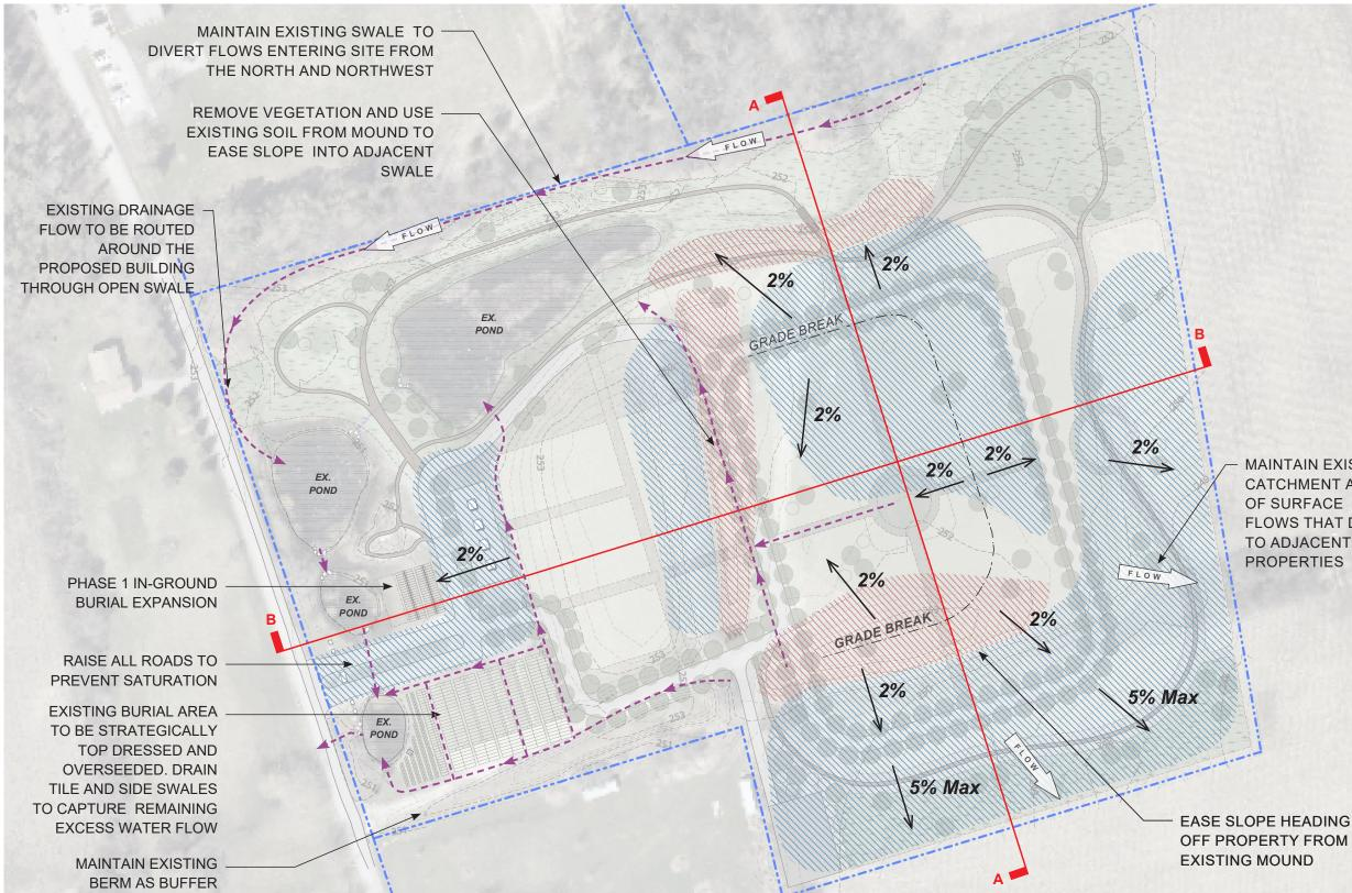
FLOW MAINTAIN EXISTING CATCHMENT AREA OF SURFACE FLOWS THAT DRAIN TO ADJACENT
