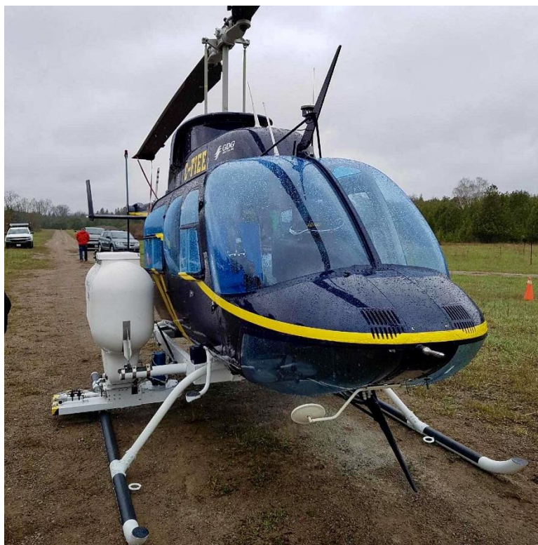
Figure 3.4 GDG Aviation – Bell helicopter equipped with Simplex spreading system used in Georgina
