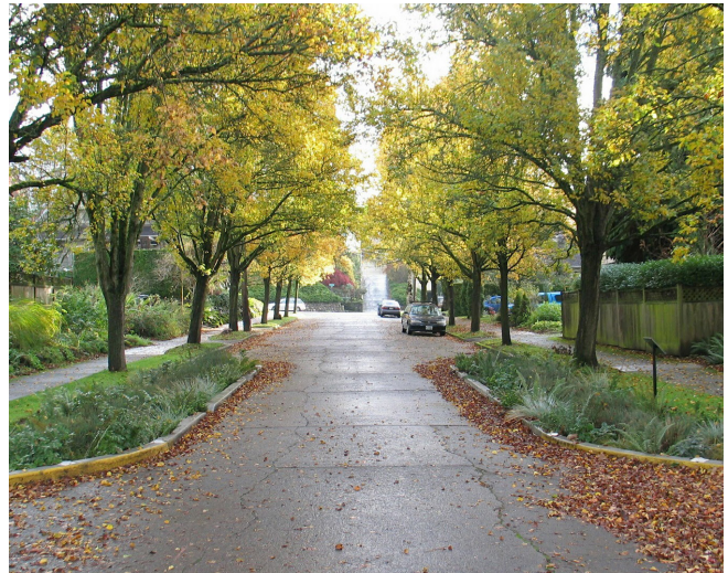
Bioswales in the public right-of-way to improve infiltration.
