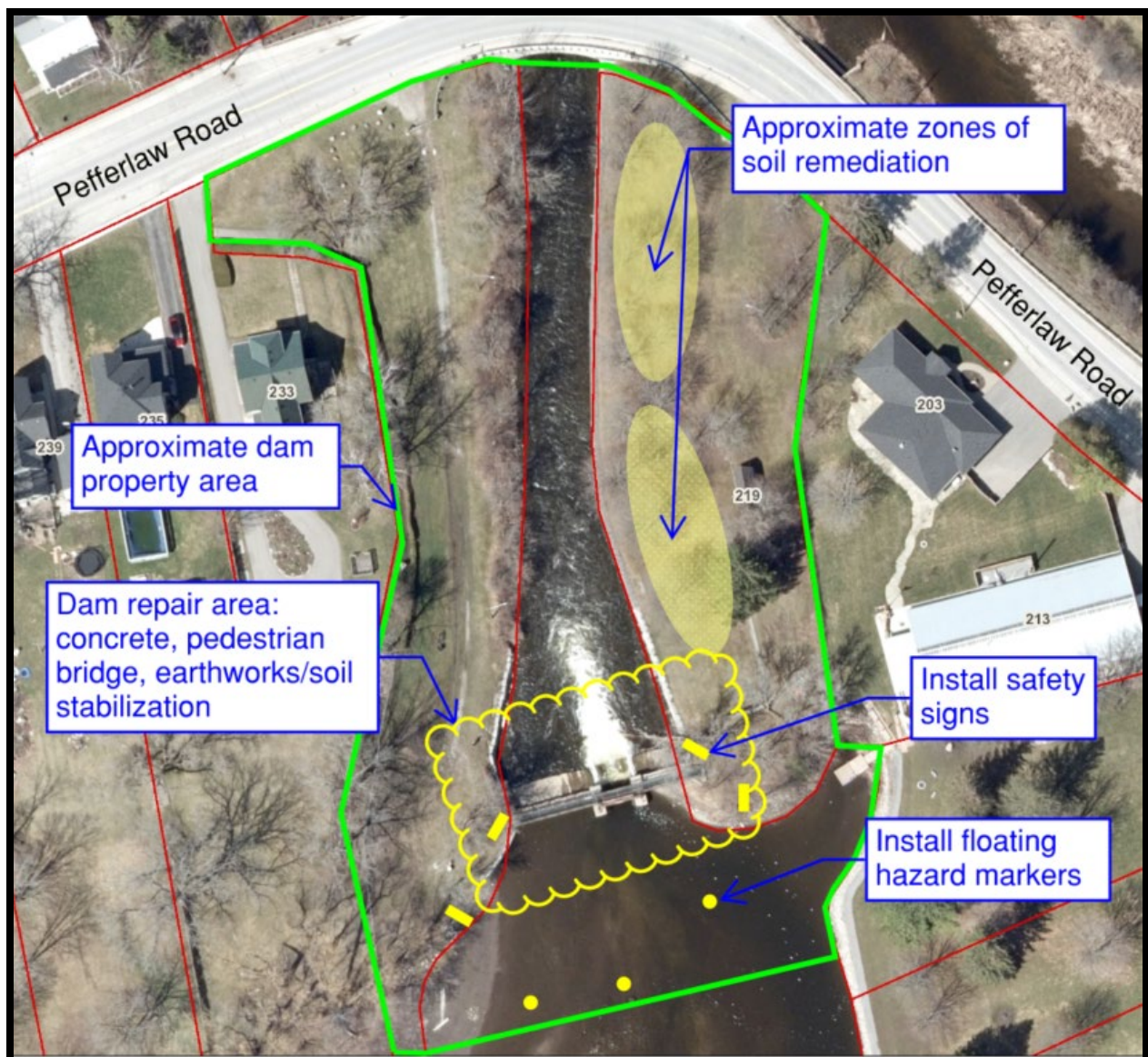
Figure 1 – Pefferlaw Dam Capital Works
