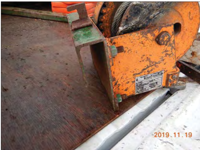
Typical Winch J-Shaped Mounting Plate/Bracket
