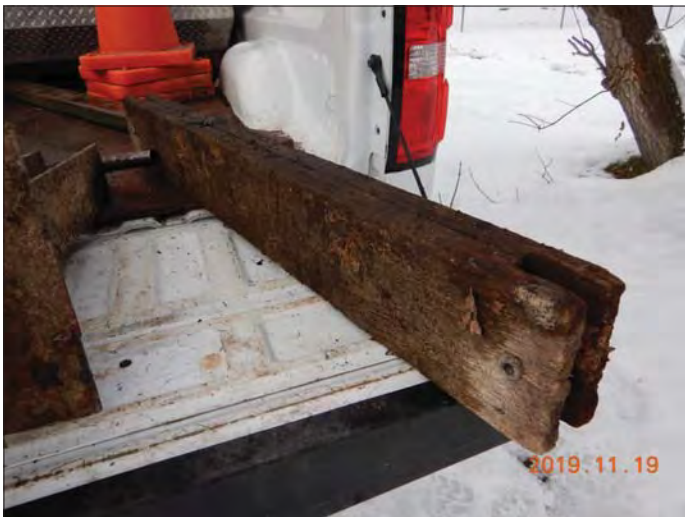
Photo 2857 - Sept 19, 2019 Pefferlaw Dam Typical Flashboard
