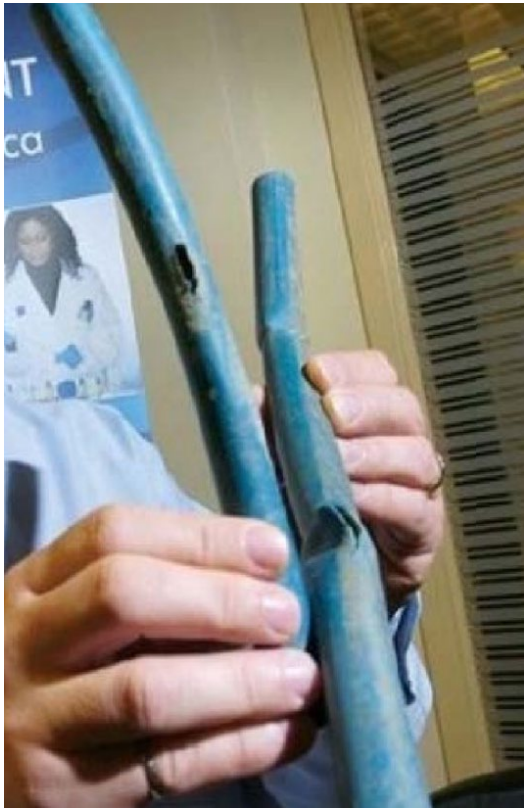
Figure 1: Deteriorated pieces of polybutylene pipe
