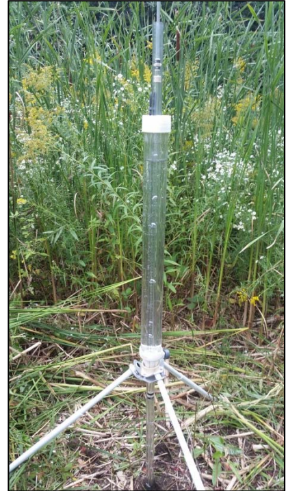
Figure 7.1: In-situ infiltration testing via Guelph Permeameter.
