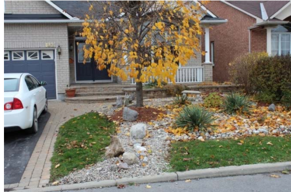
Figure 6.2: Typical Front Yard Residential Source Control.
