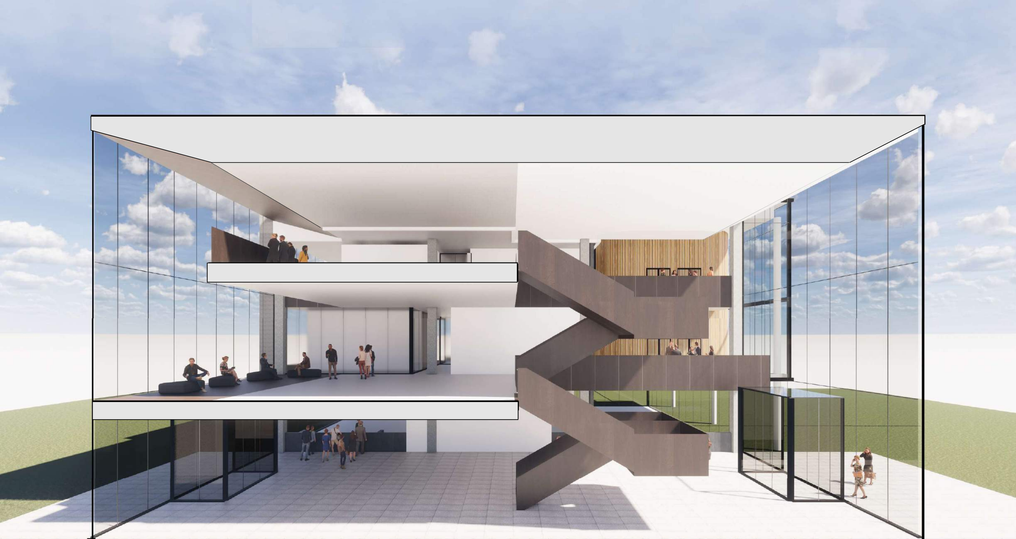
Sectional view through atrium and continuous wood ribbon feature.
